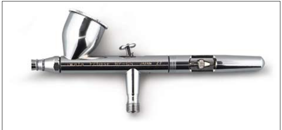
Fig. 2 Double-action airbrush. On a double-action airbrush, like this Iwata Eclipse, the air flow is controlled by pushing the trigger down; the paint flow is controlled by pulling the button back. The paint flows into the body of the airbrush from a gravity-feed cup. FineScale Modeler photo
