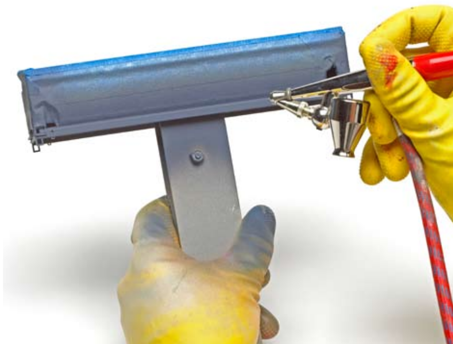
Fig. 5 Model handling. Handles, such as this one by GB Engineering, make it easier to rotate a model when airbrushing. You can also make your own handle from scrap wood or foam blocks, but use foam only with acrylic paints as organic-solvent-based paint will dissolve foam.
