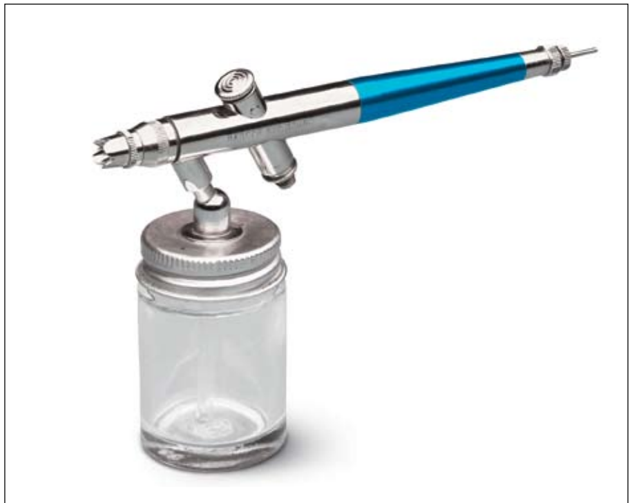
Fig. 3 Hybrid airbrush. The Badger 200 is an example of a single-action airbrush with internal mixing. The brush has the longitudinal needle found on double-action brushes, but the paint volume is controlled by turning the knurled knob on the end of the needle instead of with the trigger. FineScale Modeler photo
