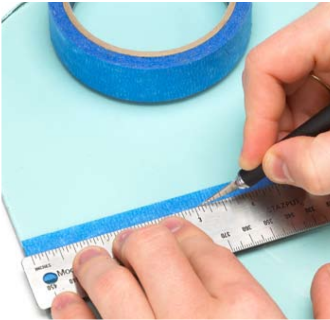
Fig. 6 Sharp separation lines. A favorite modeler's trick is to put masking tape on a piece of glass, lay a steel straightedge over it, and cut a strip using a hobby knife with a fresh no. 11 blade. Use the cut edge to mask the separation line between colors.
