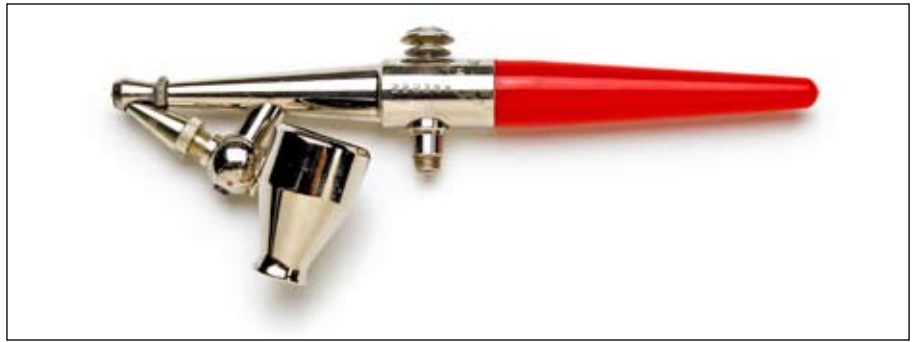
Fig. 1 Single-action airbrush. The Paasche H is an example of a single-action airbrush. With this style of brush, the air flow draws the paint up from the color cup (or bottle) into the angled paint nozzle. The knurled nozzle adjusts paint volume, and the button on the top controls the air flow.
