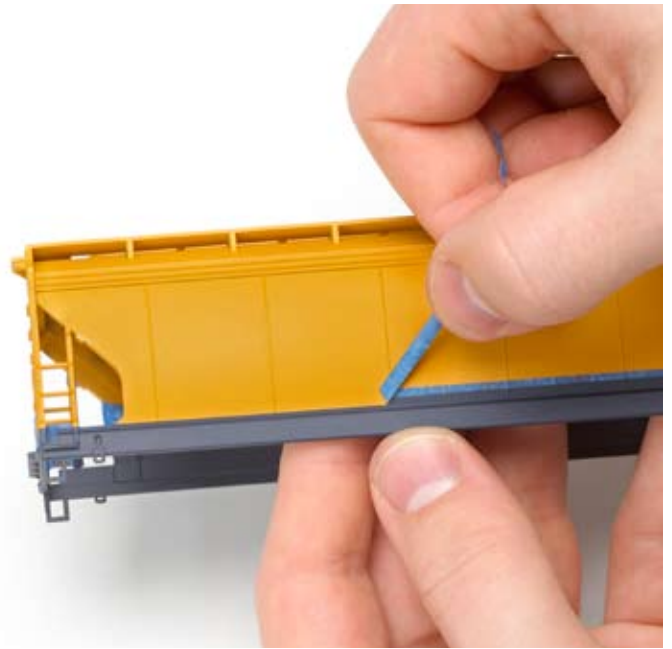
Fig. 7 Removing the mask. Even though the paint is dry, it can still peel off if you're not careful. Slowly pull the masking tape up and away at an acute angle from the last color applied. Don't leave the tape on the model too long, or it will leave residue on the model.
