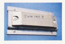
Electronic "tags" carry information about the car they are mounted on. Reporting marks, and car type and size can be "read" by scanners.
