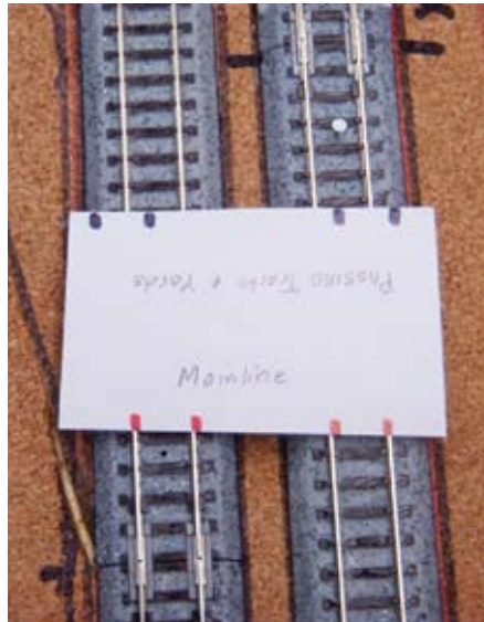
Fig. 8 Spacing guide. Dick used a notecard to maintain proper track spacing on the layout. The red marks of the main line match up with the super-elevated double track from the Unitrack V11 set.
