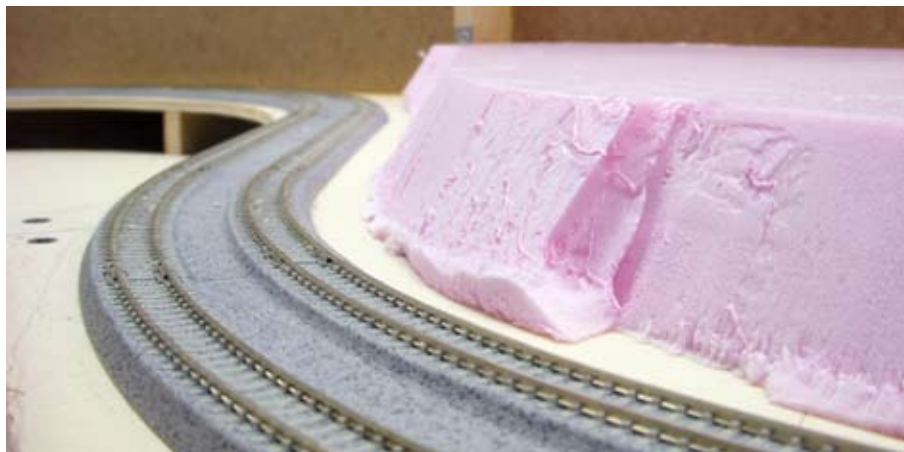
Fig. 1 Cutting foam. Dick's friend Stener Harildstad used a serrated kitchen knife to cut the extruded-foam insulation board. The sloping contour of the foam roughly matches the railroad right-of-way.
