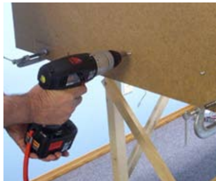
Fig. 18 More fascia. Stener attached large hardboard pieces to the ends of the layout with screws.
