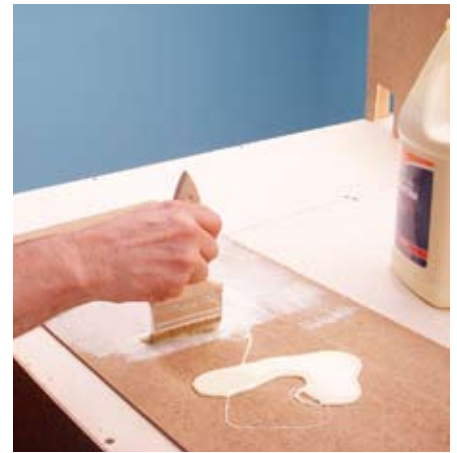
Fig. 16 Two-sided backdrop. Since the laminated backdrop couldn't be screwed together, Stener applied a liberal amount of carpenter's wood glue to the mating faces.
