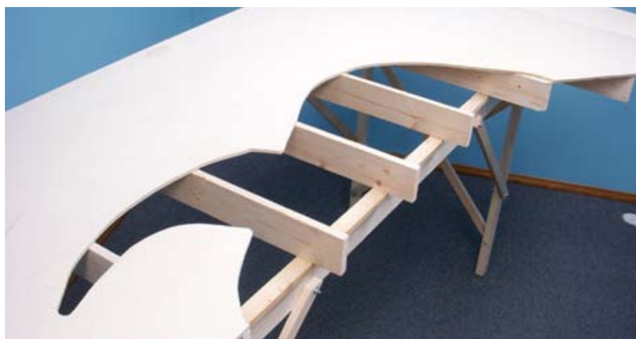
Fig. 8 Cookie-cutter benchwork. Meadow Valley Creek runs out from between a pair of canyon walls, flows beneath a through-truss bridge, and then spreads out (in flood times) into a wide wash. Stener marked this on the plywood and then cut it out, saving the cut piece for the floor of the wash.
