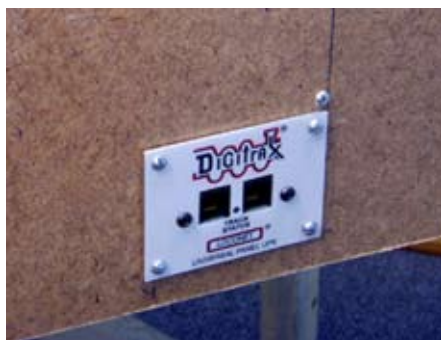
Fig. 9 Faceplate mounting. Dick used small nuts, bolts, and washers to secure the faceplates.
