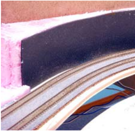
Fig. 3 Tunnel linings. Before enclosing the tunnel, Dick lined the walls with Woodland Scenics Track-Bed.
