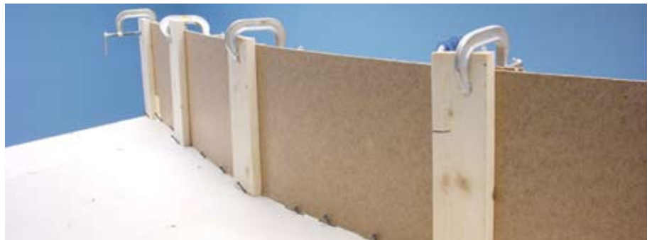
Fig. 17 Squeezed together. C-clamps at the top of the backdrop and drywall screws at the bottom force the back-to-back pieces (rough side to rough side) of tempered hardboard together until the carpenter's glue dries.
