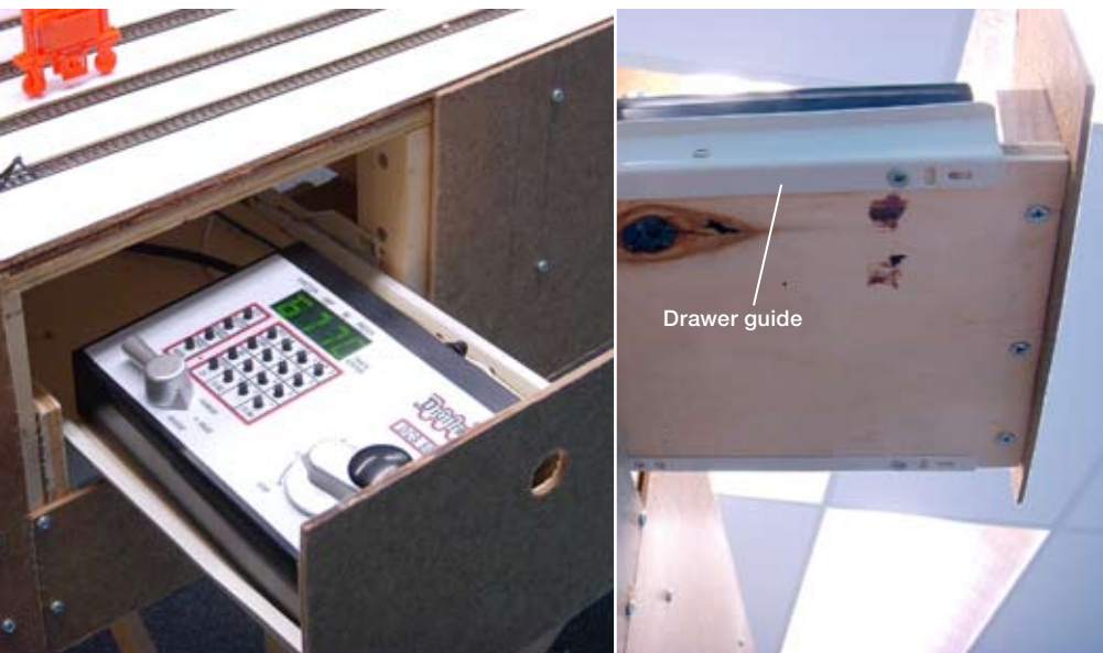
Fig. 4 Control drawer. The command station drawer is inset into the fascia. Dick made it using scrap material and drawer slides.
