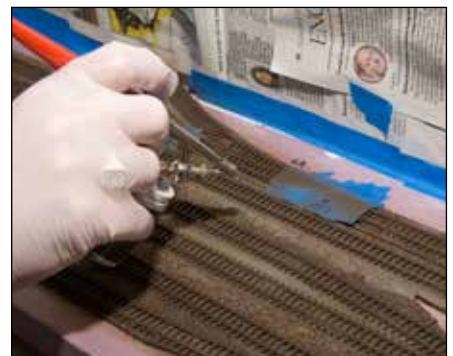
Fig. 24 Painting the track. Once laid, the track was airbrushed rail brown; turnouts were colored by hand with a paint marker.
