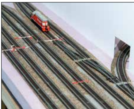
Fig. 22 Colorful trackwork. Jumpers connect the staging tracks; they were later painted to match the track and surrounding terrain.
