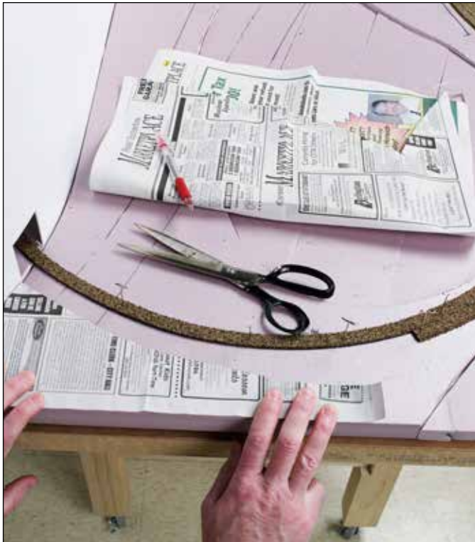
Fig. 12 Paper templates first. To get a good fit in elevated scenery areas, we made paper templates and then transferred them to foam pieces.
