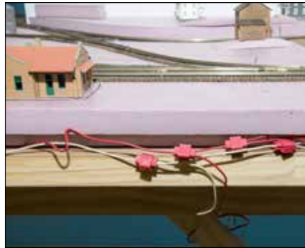
Fig. 20 Bus lines and suitcases. The feeders connect to the bus lines in the trough between the foam layers along the outside of the layout.
