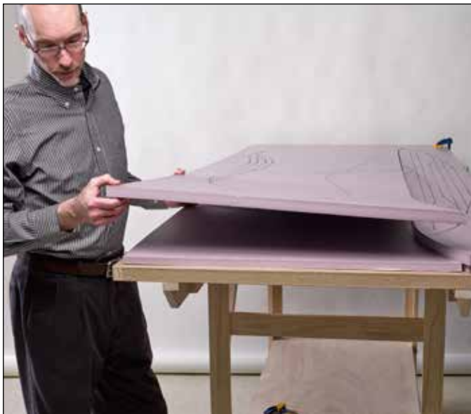
Fig. 7 Two sheets of foam. David Popp used two sheets of foam board for the surface of the layout, with the lower piece cut smaller to create a wiring trough.
