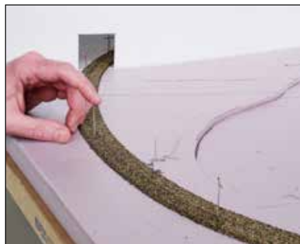
Fig. 16 Holding cork in place. We used metal T-pins to keep the roadbed curves from moving as the glue dried.
