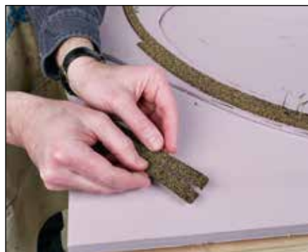
Fig. 14 Splitting the roadbed. Using split roadbed allows the strips to conform to curves without buckling.
