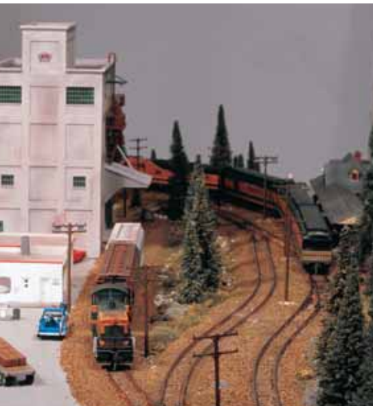
4. Unfettered by the arriving passenger train, the crew of GN SW9 no. 16 continues switching at Centennial Mills. A double-loop track plan, divided into 10 electrical blocks, makes it possible to operate two trains independently.
