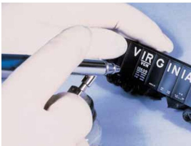
▲ Fig. 3 RIBBED SIDES. When spraying light streaks on rib-sided cars such as this hopper, John aims the spray between the side posts. Starting at one end, he uses a quick top-to-bottom motion to spray each car panel individually.
