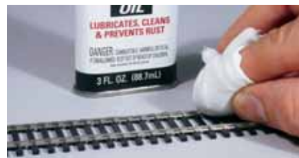
Fig. 2 OILING RAILHEAD. Applying a light coat of oil with a piece of soft cloth makes it easier to remove the paint later.
