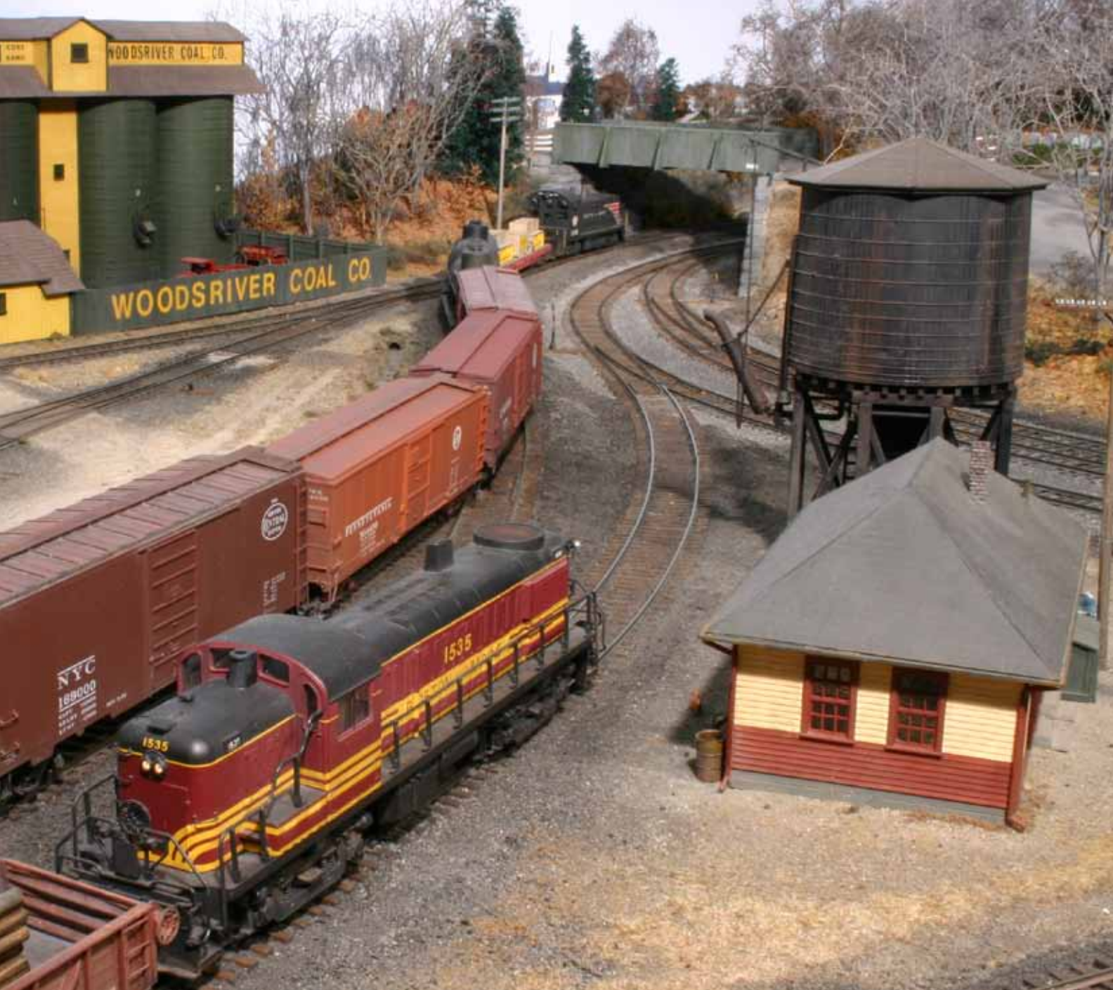
Fig. 3 Yard lead. The Woodsriver Yard lead is a separate track that runs parallel to the main line so switching can continue as other trains arrive and depart. The train in the foreground is departing to the south. Over the hood of the 1535 is the crossover connecting the lead and arrival/departure tracks. The yard office is also located along the lead.
