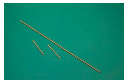
Brass studding rod used to make long bolts
