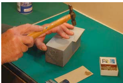
Adding rivet detail
