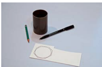
Boiler front marked out round Tube and cutting lines added
