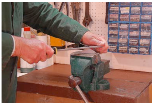
Filing the boiler front to fit the boiler diameter
