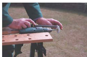
With a 1/4" bolt through it's centre and gripped in the drill chuck the desired diameter disc is achieved.
