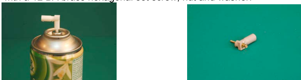
Steam sand feed unit fabricated from air freshener nozzle.
