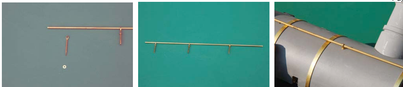
Formation of handrails from brass rod, split (cottar) pins and washers.
