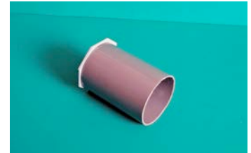
Outer disc waiting to be filed to boiler outside diameter.
