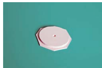
Inner disc with outer front waiting to be turned.
