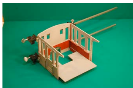
Walls held in place whilst floor is slid into position.
