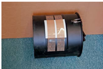
Forming curve of cab roof using a barrel and heat gun.
