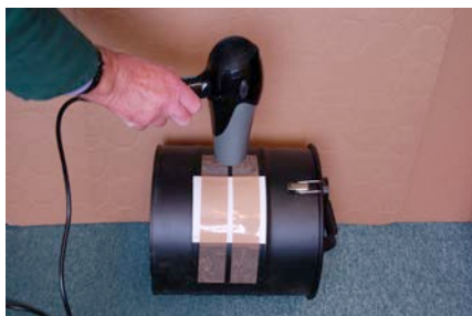
Forming curve of cab roof using a barrel and heat gun.
