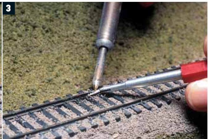
The heat-shrink tubing has been slipped over the joint and is being shrunk by rubbing the warm side (not tip) of the iron on all sides.
