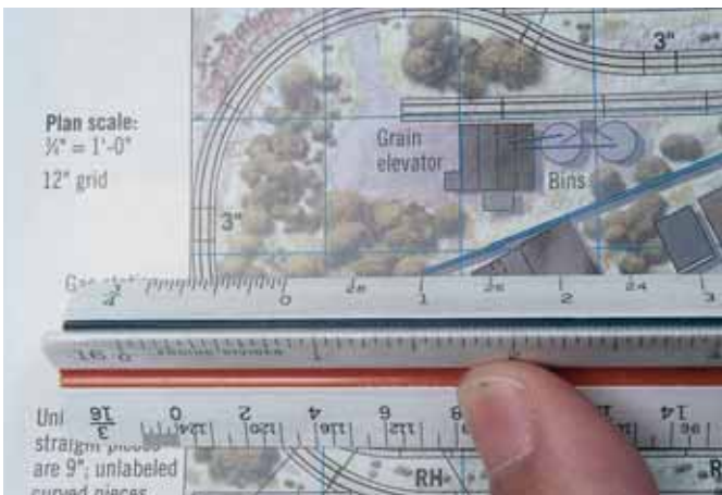
Fig. 4 USING AN ARCHITECT'S SCALE. An architect's ruler is handy for measuring published track plans. In this case the scale of the drawing is \frac{3}{4} " to the foot.
