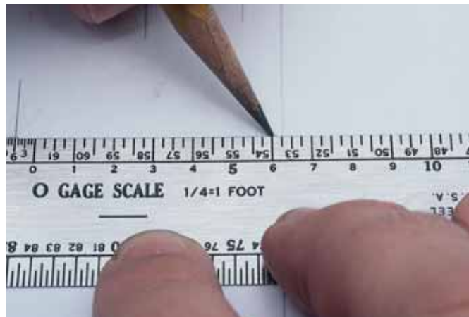
Fig. 1 TRANSFERRING DIMENSIONS. After reading the prototype dimensions from an HO scale plan, use an O scale rule to draw the outline of a door onto styrene.
