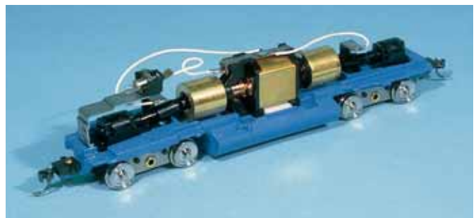
Fig. 7 NEW WIRING. Replace the original Athearn steel contact strap with flexible wires soldered in place for a more reliable electrical path.
