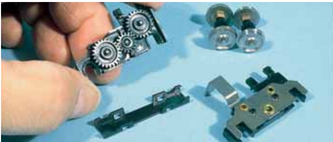
Fig. 4 GEARBOX. Be sure to clean off any molding flash (excess plastic) or dirt that you find in the gearbox.
