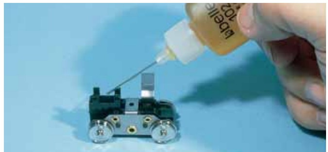
Fig. 6 LUBRICATION. Apply only a couple drops of plastic-compatible lubrication in each truck gearbox.
