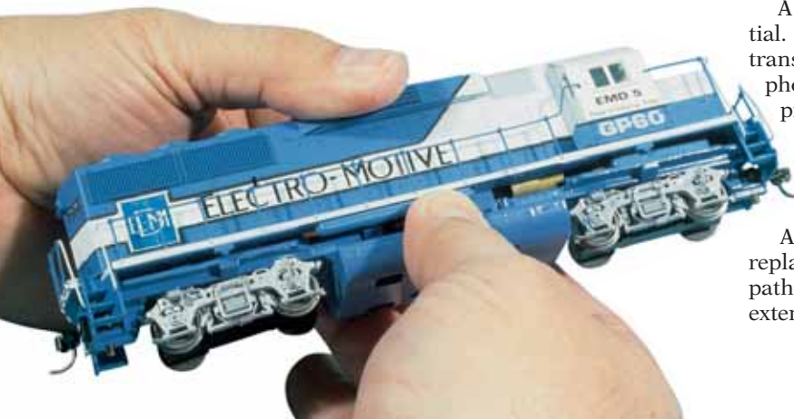
Fig. 1 REMOVING BODY. Look for side lugs or clips to determine how to remove the body.
