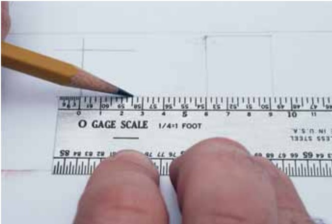
Fig. 3 CHANGING SCALES. To enlarge the window opening on the HO plan to O scale, flip the rule to O scale and measure the 30". Be sure to measure from zero, not from the end of the rule.
