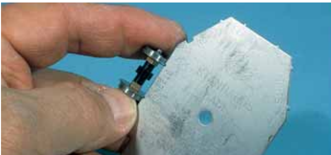
Fig. 5 GAUGING WHEELS. Use an NMRA standards gauge to check the spacing of all the wheelsets and correct any problems.
