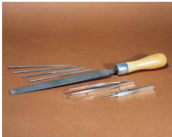
Needle files are good for cleaning out flash while the larger mill file finishes rough edges. Nonmagnetic tweezers help handle tiny parts.
