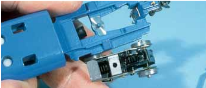
Fig. 3 TRUCK KINGPIN. Polish all electrical contact points where current is transferred between mechanical components.
