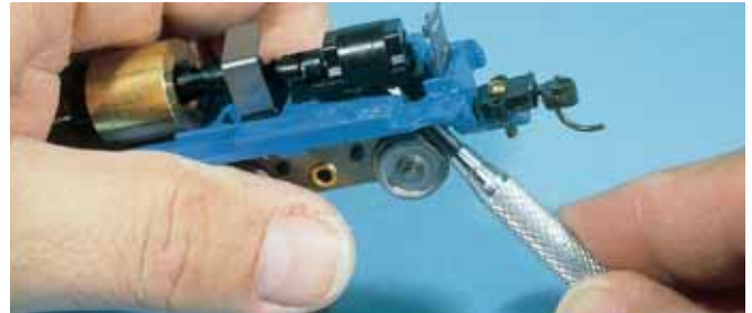
Fig. 2 REMOVING WORM HOUSING. Use a small screwdriver to gently pry off the combination worm housing and truck retainer.
