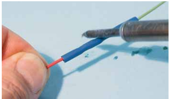
The heat-shrink tubing has been slipped over the joint and is being shrunk by rubbing the warm side (not tip) of the iron on all sides.
