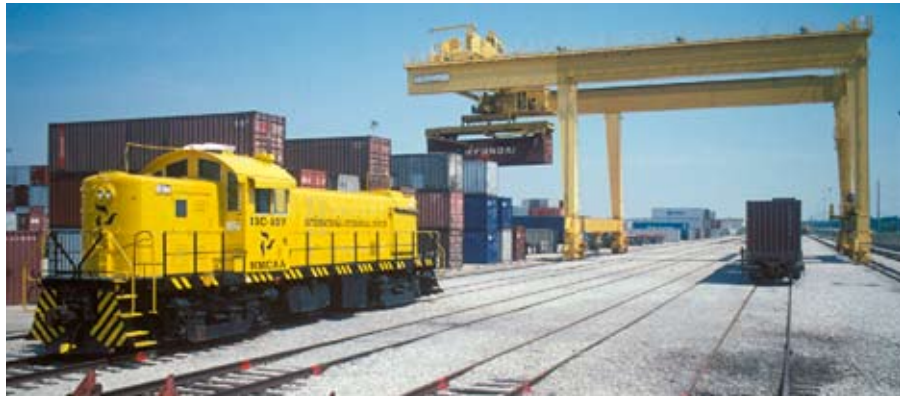
Fig. 16. The compact Huntsville (Ala.) International Intermodal Center, above and at top, is positioned between the airport runways and a small rail yard serviced by the Norfolk Southern. An Alco RS-1 handles car movements within the small yard. Its small size makes it an excellent candidate for conversion to a Layout Design Element. Bottom photo by Tony Koester
