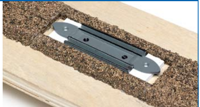
This no. 321 electromagnet is supported on white styrene blocks so the steel pole pieces are level with the top of the roadbed. The coil hangs 1\frac{1}{8}" below the \frac{1}{2}" plywood.
