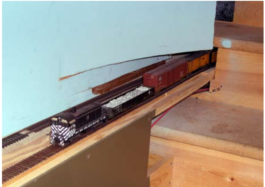
A stairway along the wall of Keith Jordan’s basement was a layout-design obstacle that proved easy to overcome. The track through the stair riser leads to a staging yard behind the stairs. Keith Jordan photo
