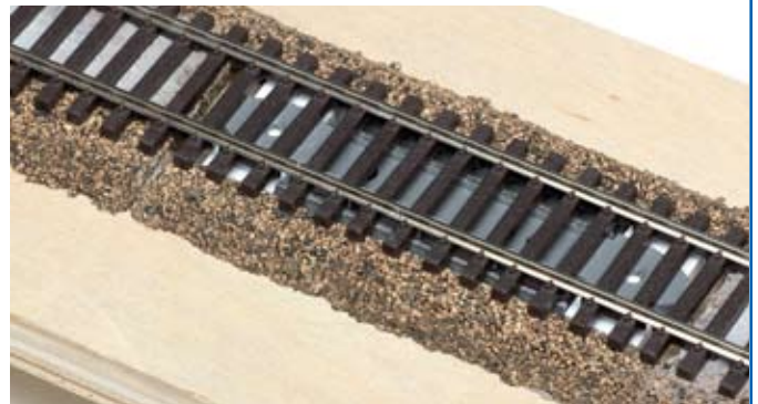
Here you can see the electromagnet's pole pieces directly under the ties. In practice you can cover the magnet opening with a piece of foil or thin paper so there won't be gaps under the ties to fill with ballast.
