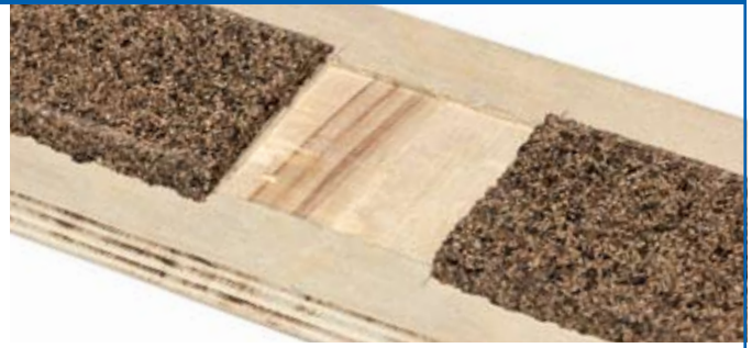
The \frac{3}{8} " thick no. 308 permanent magnet requires a recess in the subgrade so it can be level with the roadbed.
