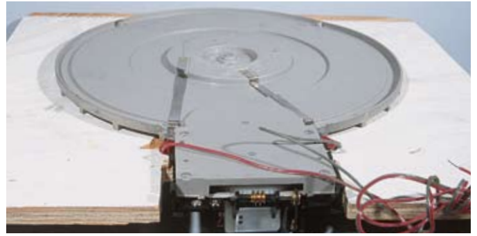
Fig. 2 Turntable mounting. This upside-down view shows the Atlas turntable mounted to the plywood base. One layer of the plywood was removed to clear the raised outer ring around the original turntable.
