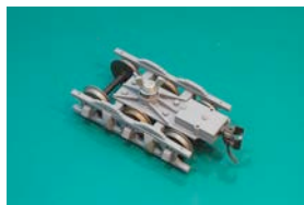
Bogie with wheels in place
