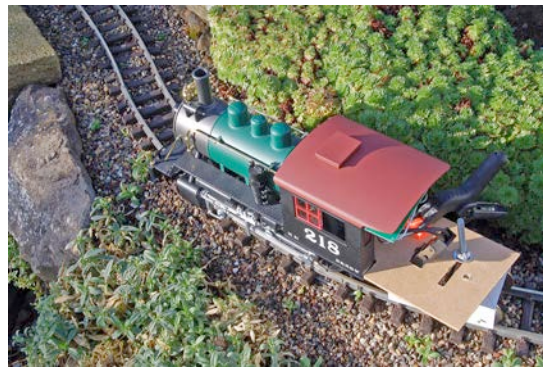
Three axle test unit on a 2'6" radius curve.
