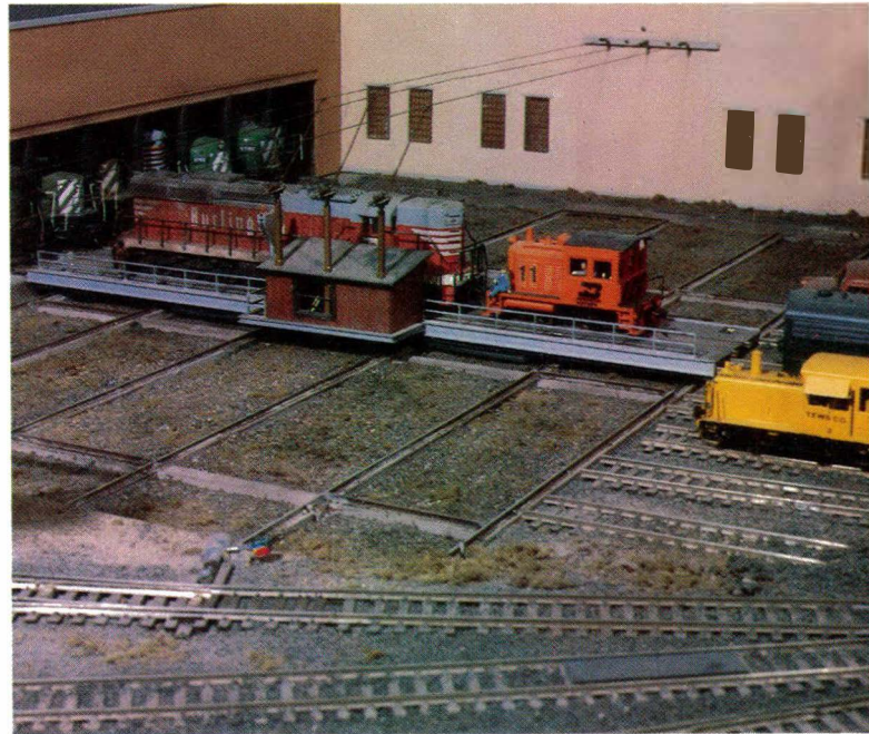
5. This rare scratchbuilt transfer table serves the locomotive and car shops of the Timber River. The table is powered by a motor hidden in the control house, and it operates from power collected from the overhead trolley wires.
