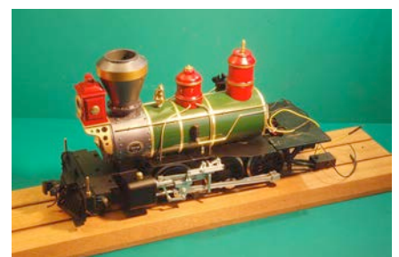
Boiler slipped over lead weight
