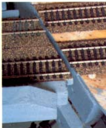
Fig. 4 ANGLED BREAKS. The rail joints at both ends are cut at an angle so they move away from each other as the gate is opened.
