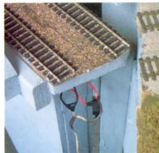
Fig. 5 POWER FEEDERS. Loops of flexible wire carry electrical power between the layout and the bridge tracks.
